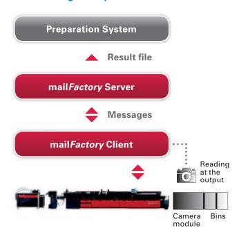
An additional reading device and a camera module are required for reading at the output. Different versions are available depending on the printed barcode type and reading requirements:
