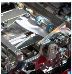
The Kern 3600 is capable of handling all formats with a maximum capacity of 27,000 inserts per hour. The continuous speed adjustment enables optimal alignment with processing conditions.
