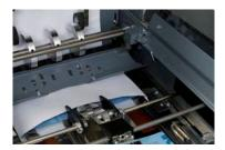
The KAS unique insertion system positively guides the material into the envelope.
