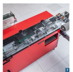
The built-in logic decides – on an application-specific basis – whether a document or document group should be rotated (both directions possible) so that it can be correctly inserted to the envelope according to window position.
